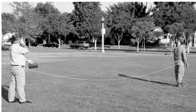
Fig. 4.73 Pipeline CP fault testing with Pearson-type detector. (Photo courtesy of Tinker & Rasor.)
