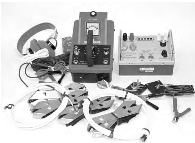
Fig. 4.71 Instrumentation to carry out a Pearson survey. (Photo courtesy of Tinker & Rasor.)
