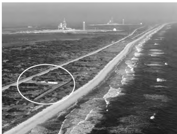
Fig. 4.80 Aerial view of the NASA Kennedy Space Center beach corrosion test site where atmospheric corrosivity is the highest corrosivity of any test site in the continental United States. (Courtesy of NASA.)
