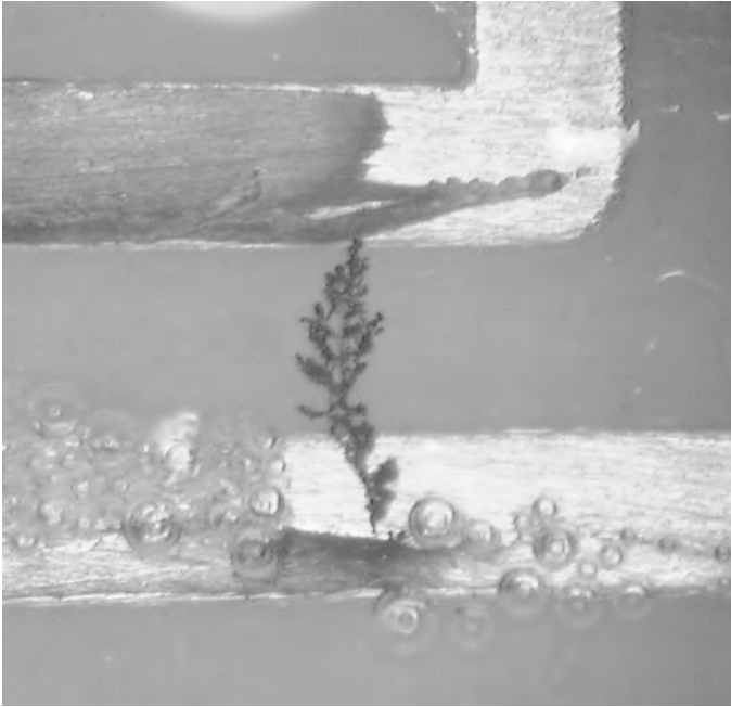
Fig. 2.3 Dendrite on a circuit board after its exposure in a test chamber. (Courtesy David A. Douthit LoCanLLC.)
