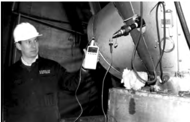
Fig. 4.1 Field corrosion monitoring using electrochemical noise recorded with a handheld data logger. (Courtesy of Kingston Technical Software.)
