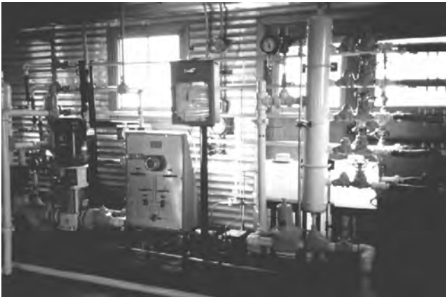
Fig. 4.17 Oil recovery microbial test lines to evaluate biocide programs. (Courtesy Kingston Technical Software.)
