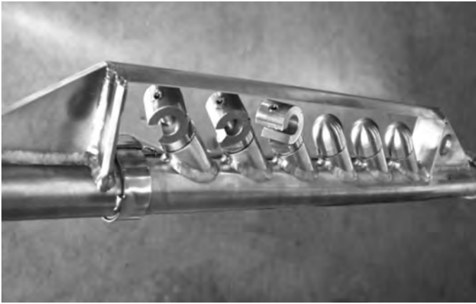
Fig. 4.7 Detail of the Hanford site 25 -cm 2 bullet and 47 -cm 2 C-ring channel electrodes. (Courtesy of Glenn Hedgemon, HiLine Engineering & Fabrication.)
