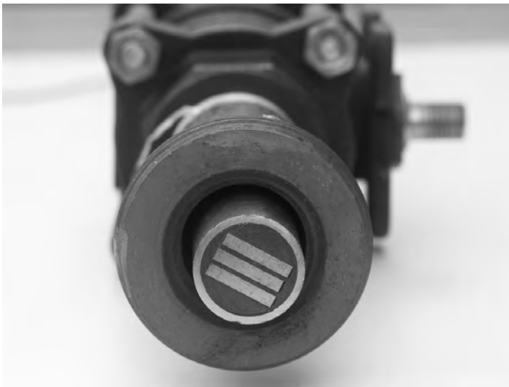
Fig. 4.45 Close-up of corrosion sensing elements used for thin-film corrosion monitoring. (Courtesy Kingston Technical Software.)
