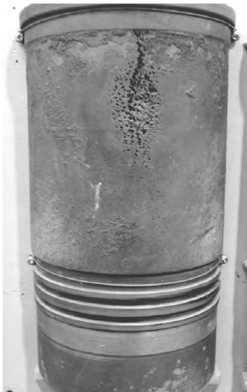
Fig. 2.18 Cavitation damage of a diesel engine piston liner on the return stroke. (Courtesy Defence R&D Canada-Atlantic.)
