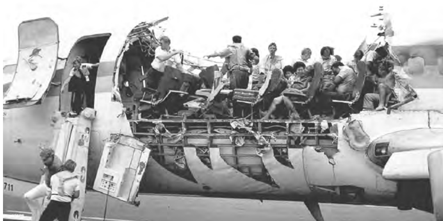
Fig. 1.11. Photograph of the Boeing 737 operated by Aloha airlines that lost a major portion of the upper fuselage in 1988.
