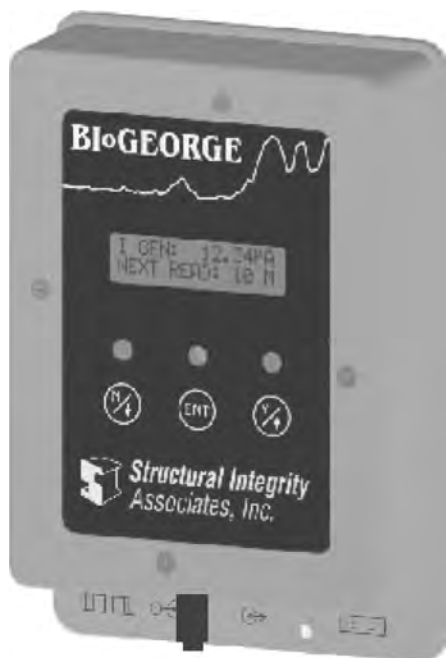
Fig. 4.68 Control box of a BioGEORGE MIC detection probe. (Courtesy of George Licina, Structural Integrity Associates, Inc.)
