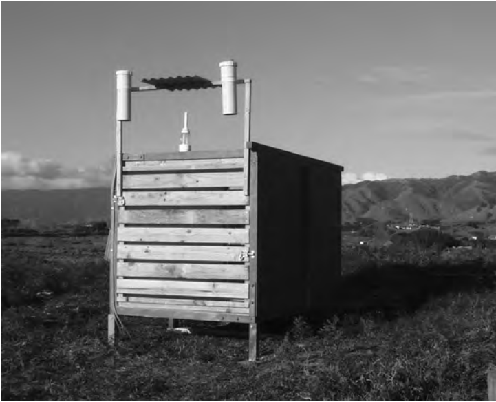
Fig. 4.78 A typical subfloor simulation box surmounted by a wet candle chloride measuring device that has been installed at several sites in Australia and New Zealand. (Courtesy of Branz, New Zealand.)
