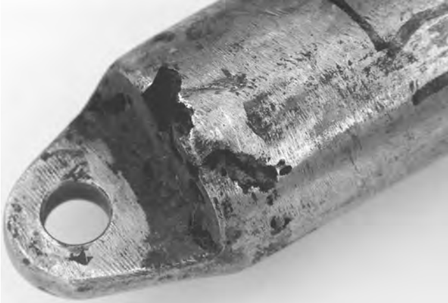
Fig. 1.18 End fitting of a welded support rod (S30300) after service in seawater. This particular stainless steel is not recommended for welding. (Courtesy Kingston Technical Software.)
