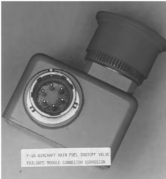
Fig. 2.2 Tin-plated pin corrosion in failsafe module connector on F-16 actuator found in the closed position with master fuel switch to master. (Courtesy David H. Horne, Hill AFB, Utah.)
