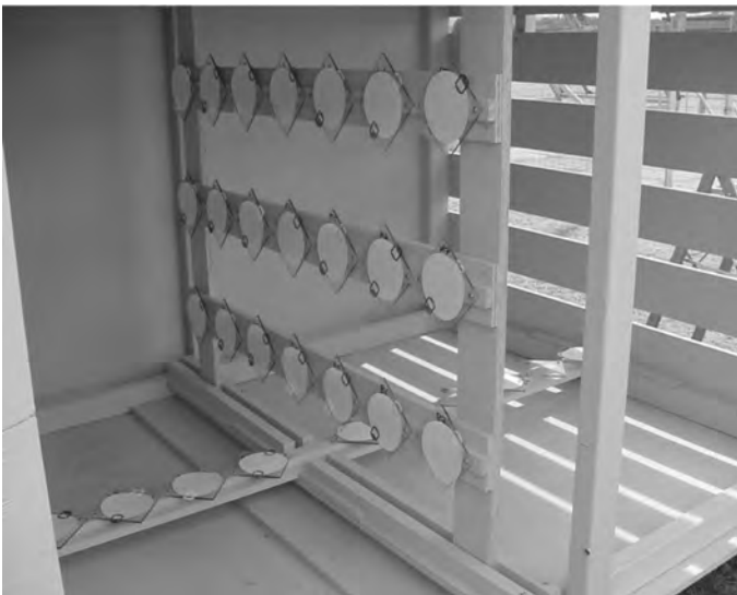
Fig. 4.79 Horizontal and vertical filter papers installed inside a subfloor simulation box. (Courtesy of Branz, New Zealand.)
