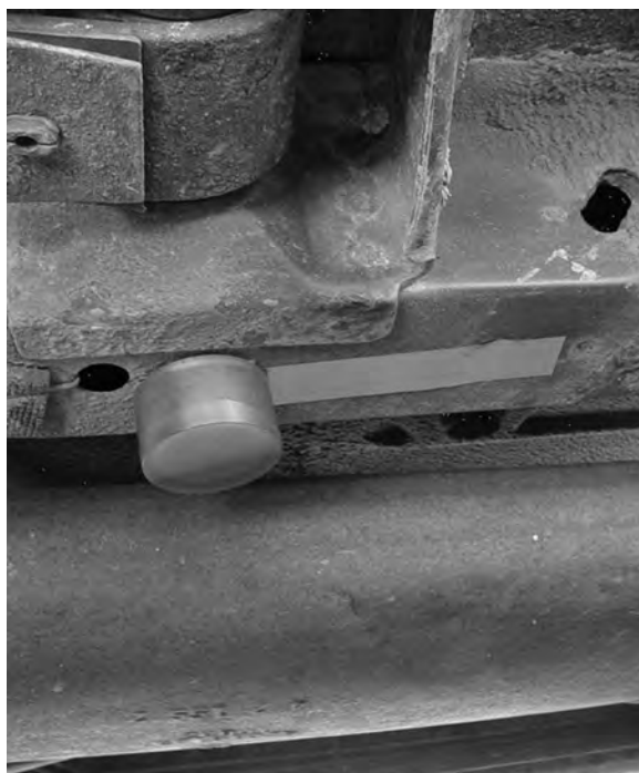
Fig. 4.43 (a) Schematic of the Coating Health Monitor (CHM) with a tape sensing element mounted on a coated metal and (b) actual sensor tape electrode and electronics housing mounted on the frame of a commercial vehicle. (Courtesy of Guy D. Davis, DACCO SCI, Inc.)
